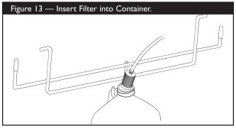
• Place the small filter end of the detergent siphoning tube into the detergent container.
