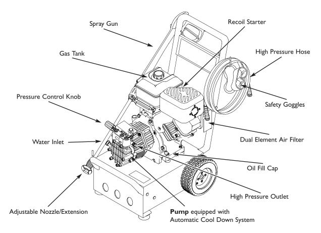
**Adjustable Nozzle/Extension** — Always attached to nozzle extension. Pull back for high pressure or push forward for low pressure; turn clockwise for narrow spray or turn counterclockwise for fan spray.
